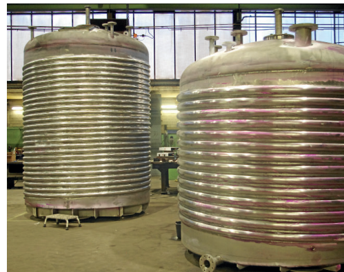
Mixing tanks from LOHSE are manufactured for example using the high-temperature nickel-chrome-molybdenum alloy 2.4605, which is also resistant to chemicals.
