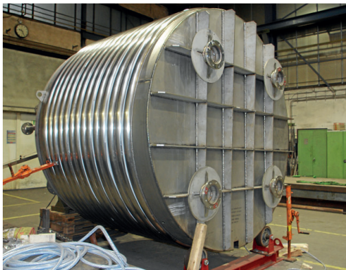
Mixing tanks from LOHSE are manufactured for example using the high-temperature nickel-chrome-molybdenum alloy 2.4605, which is also resistant to chemicals.
