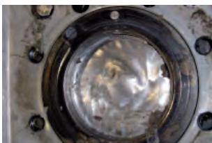
Wear of the slide plate
