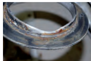
Wear of the flange ring
