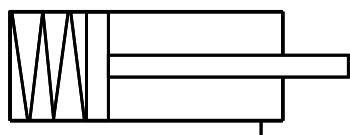
When not pressurised, the cylinder rod is fully extended.
