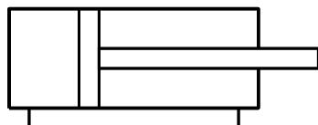
LOHSE PZ pneumatic cylinders are equipped with a fixed stop in closing direction (no adjusting nut). In opening direction, their stroke can be adjusted by means of the adjusting screw.
